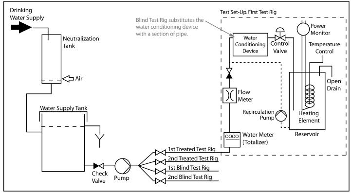
The test set-up consists of four identical sets of equipment (Two "treated" test rigs and two "untreated or "Blind" test rigs) for the examination of one type of water conditioning device. The four sets of equipment for testing are to be operated simultaneously, where two test devices are run as treated test rigs and two are run as untreated or blind test rigs.
